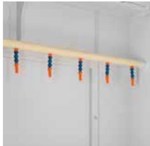
Chip shower Chip shower pipes are located at the upper section inside the machine for more efficient flow, and flexible shower nozzles can be directed to the side of the machine cover or sections where chips tend to accumulate.
