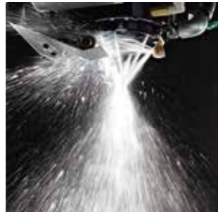
Tool washing, air-assisted type High discharge pressure and flow rate efficiently remove chips attached to the holder. Equipped with a filter clog warning function.
