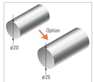
**$\phi 20$ mm max. bar as standard;  $\phi 25$ mm as option**
